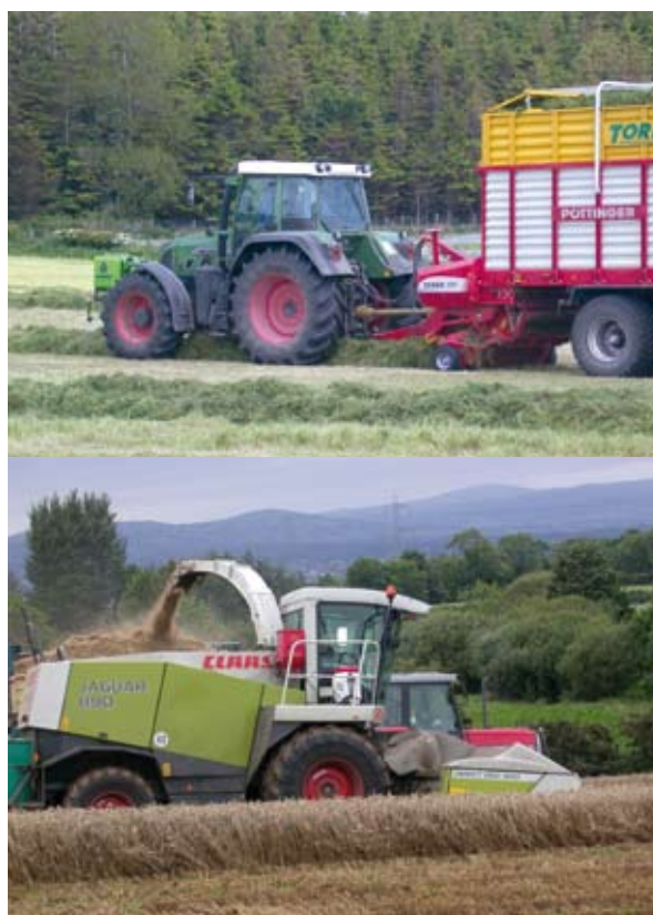
Photo 2: Grass harvesting with a self-loading forage wagon and whole crop wheat harvesting with a self-propelled forage harvester
